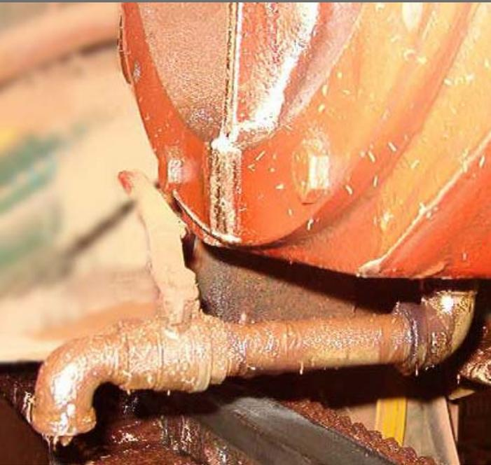
Sampling gearboxes from dead leg pipes produces erratic and misleading oil analysis results.
