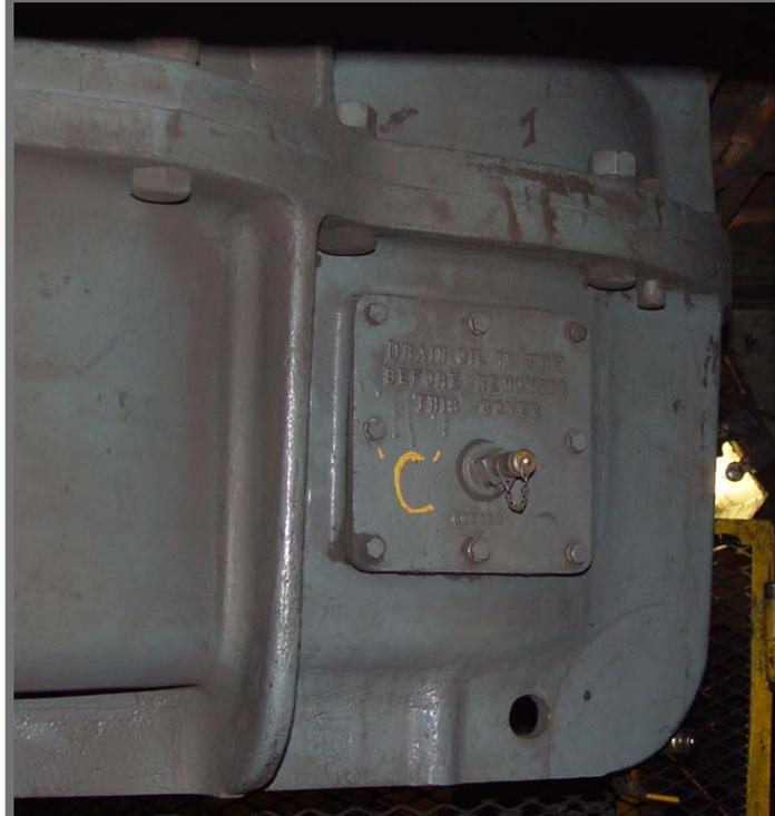
A Pitot tube provides the optimal method for sampling a gearbox.
